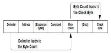
Figure 2.0: Wireless HART framing
