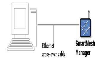
Figure 4.1: connection of manger to computer
